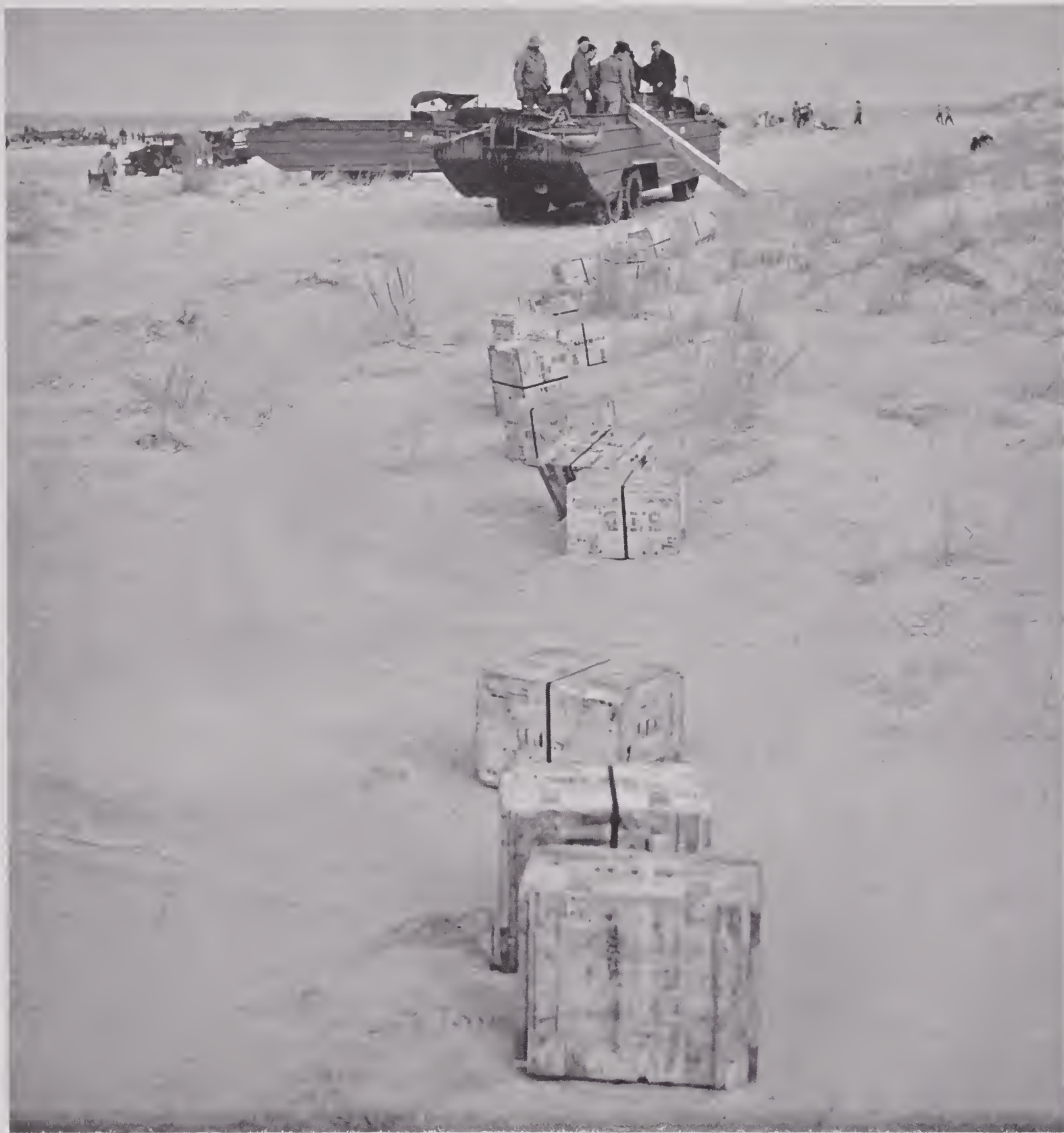
FIGURE 102. DUKWs bring cargo directly from ship through surf up to dump. Cargo is discharged by means of "hog trough" while DUKW is in motion. (In this demonstration, DUKWs landed about 30 tons in 20 minutes.)
